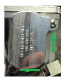
3. Once the low profile manifold is installed, reinstall the factory water manifold bolts (green arrows) and torque them to 14 N-m. Outlet and inlet ports require 10 AN o-ring fittings. Please lube all o-rings on all fittings before assembling. Top ports are outlets (hot coolant) and bottom ports are inlets (cold coolant). Plumb the system in whatever manner suits your build.
